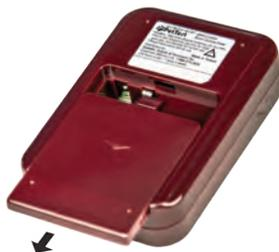
1. Place one or two thumbs on the battery cover and slide the cover down to remove.
