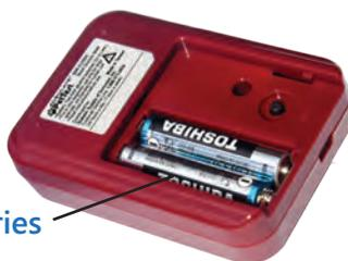
2. Remove the old batteries and replace with two new 1.5V AAA alkaline batteries, paying attention to the ⊕ and ⊖ orientation of the batteries (depicted underneath).
